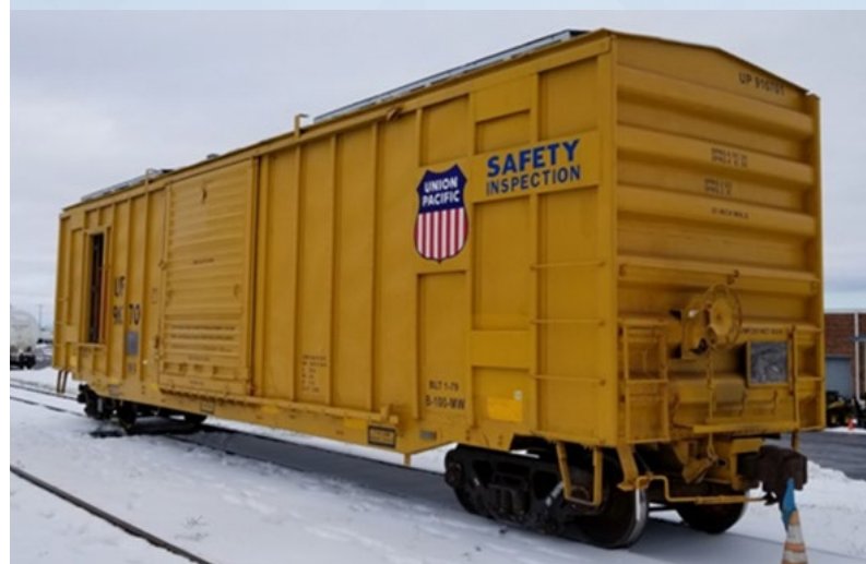
Custom-developed boxcars aid track inspection.
