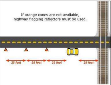
NOTE: In some cases, (because of State or Local requirements) workers may be required to carry and use 7 cones with reflective collars for flagging protection.
