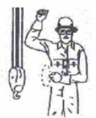
Travel: (one track crawler cranes) Lock the track on the side indicated by the raised fist, and travel opposite track in direction indicated by circular motion of other fist rotated vertically in front of body.
