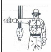
Raise Boom and Lower the Load: With arm extended, thumb pointing up, flex fingers in and out as long as load movement is desired.
