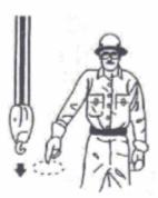
**Lower:** With arm extended downward, forefinger pointing down, move hand in a small horizontal circle.
