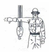
Lower Boom and Raise the Load: With arm extended, thumb pointing down, flex fingers in and out as long as load movement is desired.
