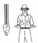
Extend Boom: (telescoping booms) Both fists in front of body with thumbs pointing outward.
