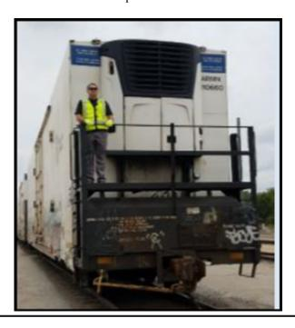
Note: Employees may transition to or from the side of equipment when the equipment is equipped with two vertical handholds (approximately shoulder width apart) or a horizontal handhold positioned to allow an erect body position when getting on or off moving equipment per Rule 81.4.2. Speed must not exceed walking speed (no more than 4 mph) when transitioning to or from side of equipment.
