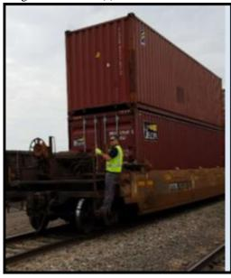
Employees may ride on the deck of an empty flat car only if it can be mounted safely while stopped, and must kneel or sit as near as possible to the center of the car until the car has come to a complete stop.
