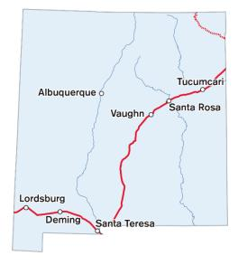
The east-west lines and the north-south lines in New Mexico converge at Santa Teresa, home to Union Pacific's 2,200-acre intermodal ramp and refueling station. Employing state-of-the-art technologies, the facility allows the secure and efficient transference of shipping containers from train to truck. Completed in 2014, the \$470 million project is a catalyst for additional economic development, including warehouses, trucking and logistical distribution centers.
