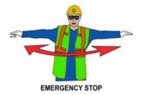
This hand signal shall be used at any time there is an unsafe condition, such as a detachment failure between the cargo container and the chassis, to immediately halt crane operations. Continue using the hand signal until you hear an acknowledgement over the loudspeaker.
