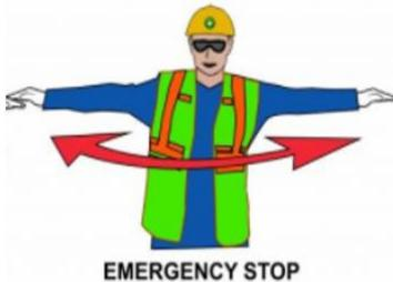
This hand signal shall be used at any time there is an unsafe condition, such as a detachment failure between the cargo container and the chassis, to immediately halt crane operations. Continue using the hand signal until you hear an acknowledgement over the loudspeaker.
