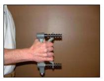
Employees need to grip and utilize manual cutters when cutting wire. Applicants must demonstrate the ability to generate the required force to accomplish this task. During this test, applicants will grip a testing device with each hand separately.
