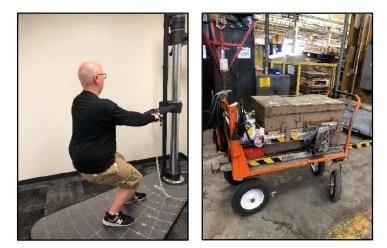
Employees are required to pull carts and other mobile objects. During this test, applicants will pull a testing device towards the body to demonstrate the ability to generate the force required to accomplish this task.
