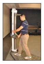
Applicants must be able to switch track junctions to redirect a train. This task is performed by pulling up on and rotating an ergo switch from the locked position. Applicants must demonstrate the ability to apply sufficient force to the switch by pulling towards their bodies in an angled direction on the testing device.
