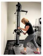
Applicants must be able to switch track junctions to redirect a train. This task is performed by pushing an ergo switch into the locked position. Applicants must demonstrate the ability to apply sufficient force to the switch by pushing away from their bodies in an angled direction on the testing device.
