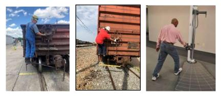
Setting the wheel brake on a train car prevents the movement of cars on a track. Applicants must demonstrate the ability to apply enough force to set a wheel brake. A device is used to simulate the body position required when performing this task and measures the amount of force applied. The force is applied as an outward pull.
