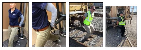
Employees must demonstrate the ability to apply the required amount of force to align a draw bar on the back or front of a train car. An upward lift force is measured as the applicant lifts on the calibrated apparatus as shown in these two pictures.
