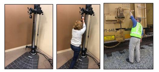
Employees are required to perform specific job tasks on specialty train cars such as those carrying automobiles. Setting the brake on an auto rack is completed with an upward push. Applicants must demonstrate the ability to apply enough force to set the auto rack brake by pushing up on the testing device.
