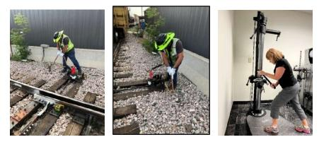
Applicants must be able to switch track junctions to redirect a train. This task is performed by pushing an ergo switch into the locked position. Applicants must demonstrate the ability to apply sufficient force to the switch by pushing away from their bodies in an angled direction on the testing device.
