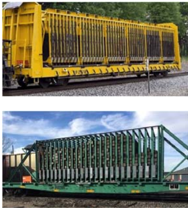
Wood Tie Unloading
