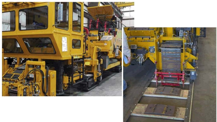
Tie Plate Distribution Automation
