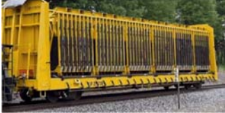
Wood Tie Unloading
