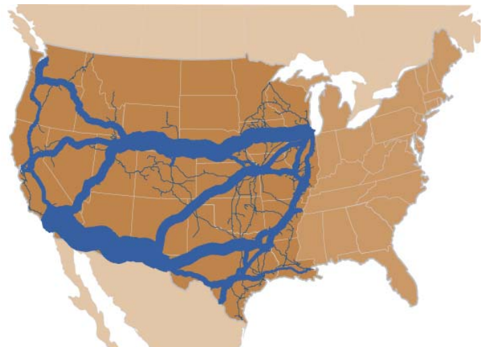
Lane density based on carloadings. Line thickness depicts traffic density.
