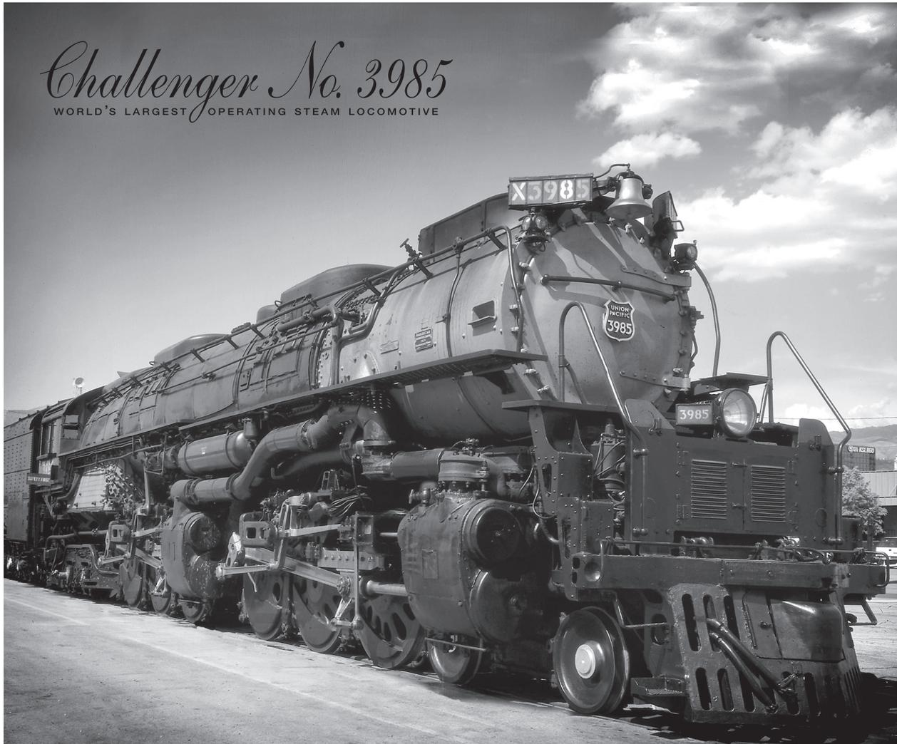
The Challenger No. 3985 was designed by Union Pacific and built in 1943 by the American Locomotive Company. It is one of 105 Challengers built for Union Pacific between 1936 and 1943 and is the only operating engine of its class in the world today – the largest and most powerful operating steam locomotive.
