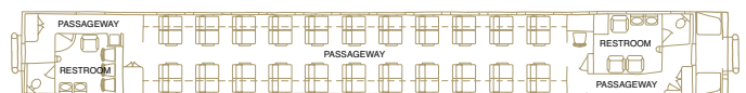
Configuration: City of Salina is a Flat Coach Car with public restrooms at each end of the car and coach-style seating in the remainder of the car. Total seating capacity is 44.
