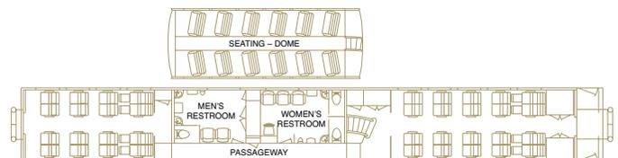
Configuration: *Columbine* is a Dome Coach Car. The short end of the car has coach-style seating for 16, and the long end of the car has coach-style seating for 20. The dome has seating for 24, giving this car a total seating capacity of 60. The car has public restrooms in the belly.
