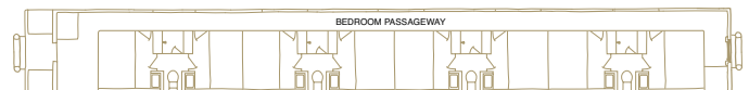
Configuration: Lake Forest is a Sleeper Car featuring four, two-room suites. The rooms are connected by the private bathroom. (Sleeps four guests)
