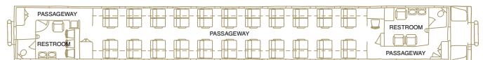
Configuration: Portland Rose is a Flat Coach Car with public restrooms at each end of the car and coach-style seating in the remainder of the car. Total seating capacity is 44.
